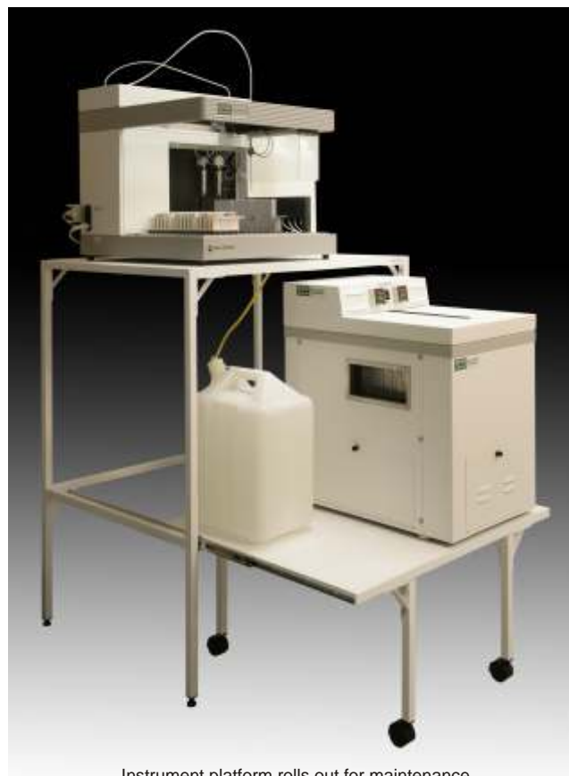
Instrument platform rolls out for maintenance.
